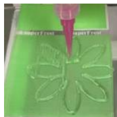
Fig. 1: 3D printing of a flower using TEMPO-CNF ink.
