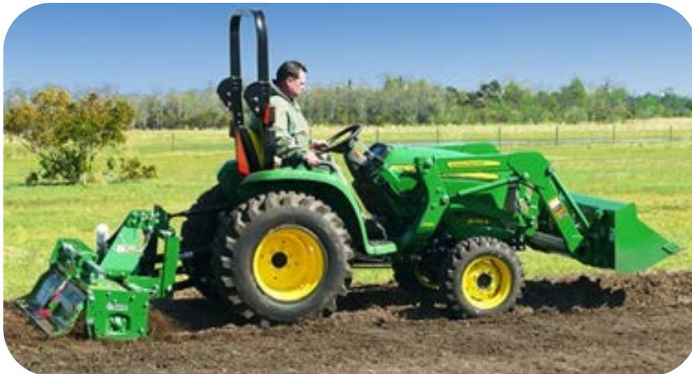
Tractor with tiller, front in loader, forks and mower.
