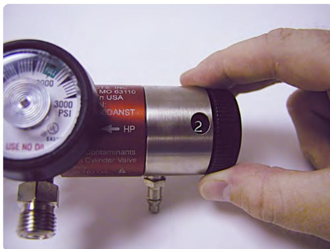
**Adapters.** In some regions, oxygen-compatible adapters accommodate various regulators with other oxygen cylinders. These adapters provide flexibility when one travels to other areas where different cylinders and valves are used. Adapters also let you use regulators designed for portable oxygen cylinders with large nonportable ones.
